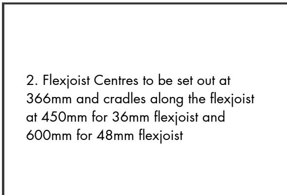
2. Flexjoist Centres to be set out at 366mm and cradles along the flexjoist at 450mm for 36mm flexjoist and 600mm for 48mm flexjoist
