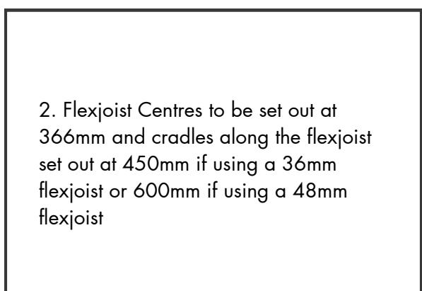
2. Flexjoist Centres to be set out at 366mm and cradles along the flexjoist set out at 450mm if using a 36mm flexjoist or 600mm if using a 48mm flexjoist
