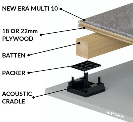
Multi Up 10 is a system that uses the Acoustic cradle and offers a higher level of impact sound isolation, whilst providing lightweight 10mm interlocking recycled rubber tiles, making it an ideal solution for ground or upper level gym and free weight areas with light activities.
