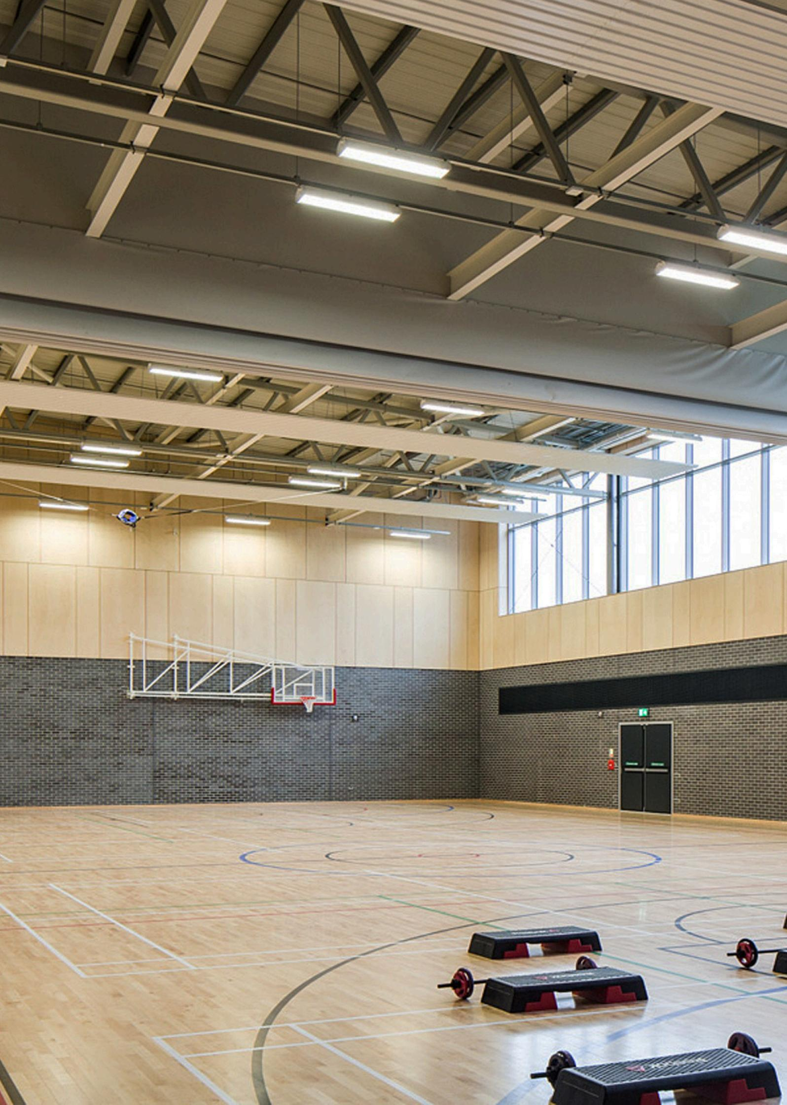
Gymflex Arena is the highest performance floor for large sports halls that require the best in area elastic standards. With a height range of 74-350mm achieved using the unique New Era sports cradles, it can overcome the most challenging of levels whilst meeting EN14904 Part A4 standard.
