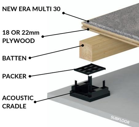
Multi Up 30 is a system that uses the Acoustic cradle and offers a higher level of impact sound isolation, whilst providing heavier 30mm interlocking recycled rubber tiles with better shock absorption, also suitable for ground or upper level gym and free weight areas for more impact use.
