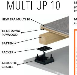
Multi Up 10 is a system that uses the Acoustic cradle and offers a higher level of impact sound isolation, whilst providing lightweight 10mm interlocking recycled rubber tiles, making it an ideal solution for ground or upper level gym and free weight areas with light activities.
