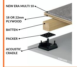
Multi Up 10 is a system that uses the Acoustic cradle and offers a higher level of impact sound isolation, whilst providing lightweight 10mm interlocking recycled rubber tiles, making it an ideal solution for ground or upper level gym and free weight areas with light activities.
