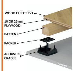
Multi Up LVT is a system that uses the Acoustic cradle and offers a higher level of impact sound reduction, whilst providing a beautiful 5mm wood effect plank LVT floor covering, making it an ideal solution for ground or upper level Studio and multi use areas.
