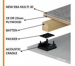
Multi Up 30 is a system that uses the Acoustic cradle and offers a higher level of impact sound isolation, whilst providing heavier 30mm interlocking recycled rubber tiles with better shock absorption, also suitable for ground or upper level gym and free weight areas for more impact use.
