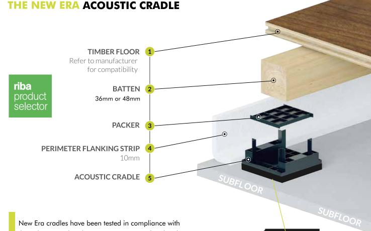
New Era cradles have been tested in compliance with the Robust Details Ltd requirements as stipulated in the Robust Detail Handbook for FFT2 resilient cradle and batten system. The minimum performance for this specification is  $rd\Delta Lw = 17dB$ . The New Era Acoustic Cradle achieved  $rd\Delta Lw = 27db$  with the minimum build up.
