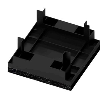
Ref L/3554/2 was with the 16/30mm cradles using a 36mm batten (average floor height 74-80mm) Result was 28db sound reduction
